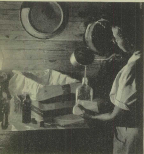
INCUBATOR is made of box and whisky bottles full of warm water. The bottles are placed at foot and sides of box, then covered with layers of cloth. This will sometimes work for as long as two or three hours.
